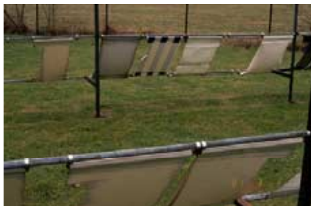
Exposition to natural weathering
