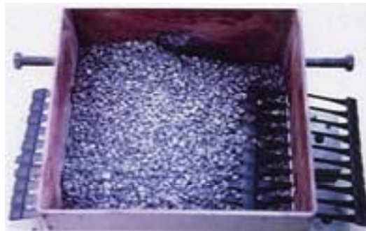
Filling Corundum into upper box
