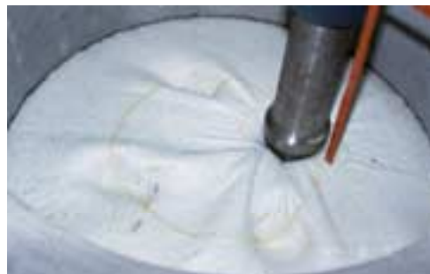
Result of drop tests – no penetration
