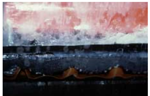
Specimen in apparatus (cusped film) top soft plate, bottom hard plate
